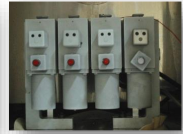
Mix test: temperature and vibrations as UIC541-08
