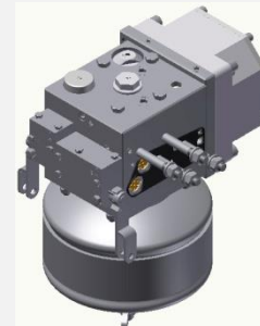
Distributor w relay valve, control chamber & aut. release
