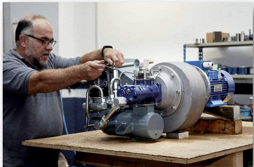
Test bench for components and brake system for RENFE high-speed trains series 103,104, 114 and 253
