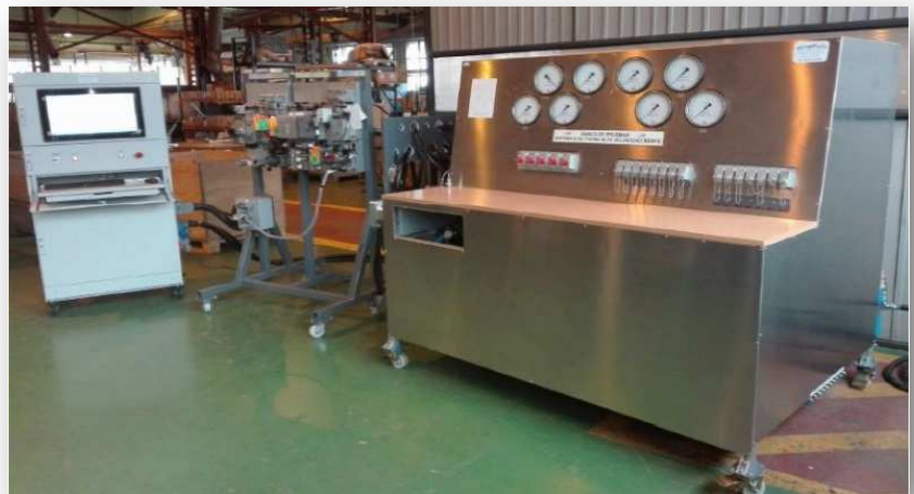
Test bench for components and brake system for RENFE high-speed trains series 103,104, 114 and 253
