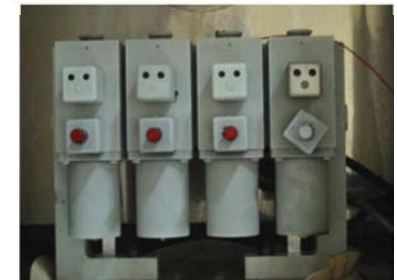
Mix test: temperature and vibrations as UIC541-08
